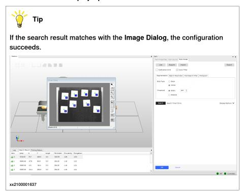
In the **Display Options** part, select **Segmentation image** to display the processed image. Select how the result will be displayed.
