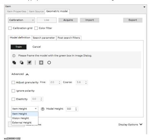
5 If the calculation method is set as Item Height, Item height: Manually enter the value for the picking/placing height.
